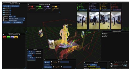
Fig. 3. The volumetric capture studio that allows for the multi-view calibration and synchronization of multiple RGB-D sensors
